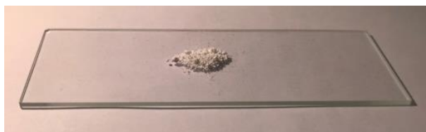
Fig. (2) The silicon nitride nanopowder extracted from thin film samples prepared in this work
