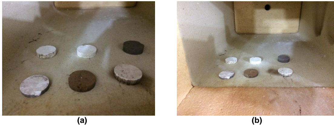
Fig. (2) Discs of prepared samples with 3-5mm thickness and 20mm diameter (in muffle furnace)
