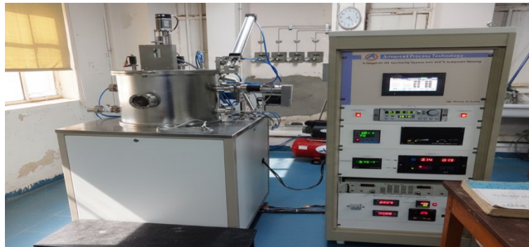
Fig. (2) RF sputtering system used in this work
