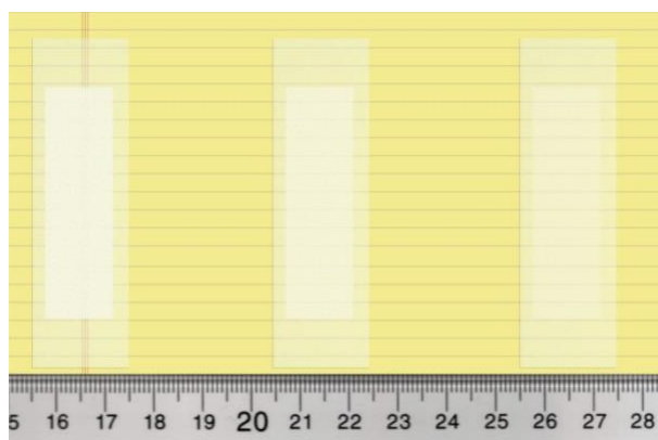
Fig. (3) The \text{Si}_3\text{N}_4 samples deposited on glass substrates at different inter-electrode distances (left to right): 2cm, 4cm and 6cm
