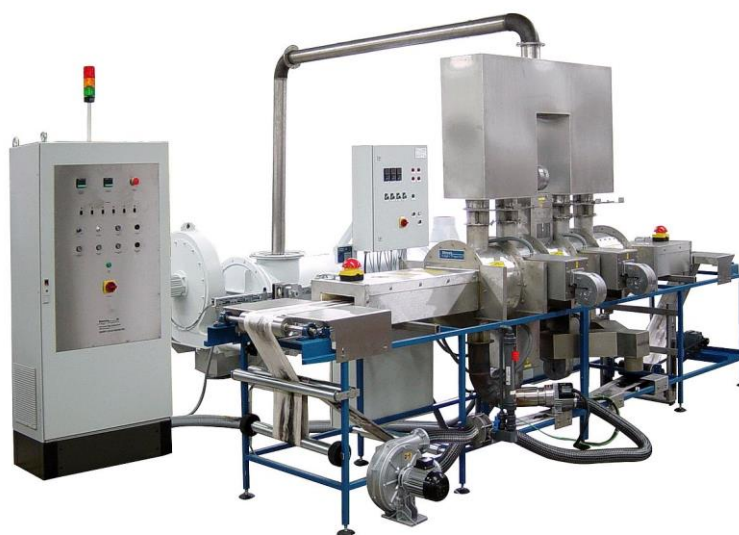
Fig. (1) Microwave furnace system used for inducing the chemical reaction in this work
