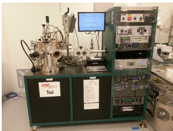
Fig. (2) The DC magnetron sputtering system used in this work
