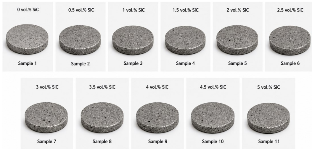
Fig. (1) The Al-Si alloy composite samples prepared in this work with different volumetric content of SiC nanoparticles
