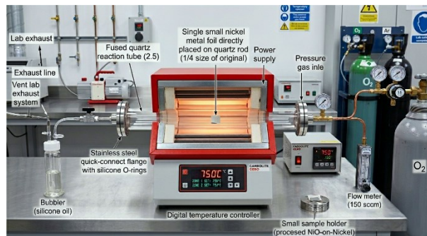
Fig. (1) The thermal oxidation/limited fusion setup to produce NiO nanostructures
