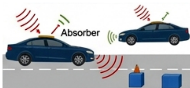
Fig. (1) The principle of the interference of the waves reflected from urban obstructions and other vehicles
